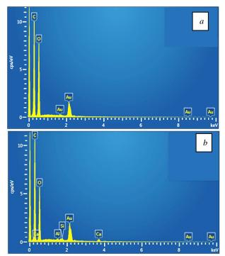
Fig. 1. EDX analysis of a) wood pulp and b) recycled waste paper cellulose fibres
