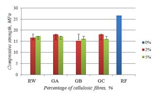
Fig. 4. Effect of cellulosic fibres content on the compressive strength of cement mortar specimens
