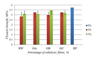
Fig. 3. Effect of cellulosic fibre content on the flexural strength of cement mortar specimens
