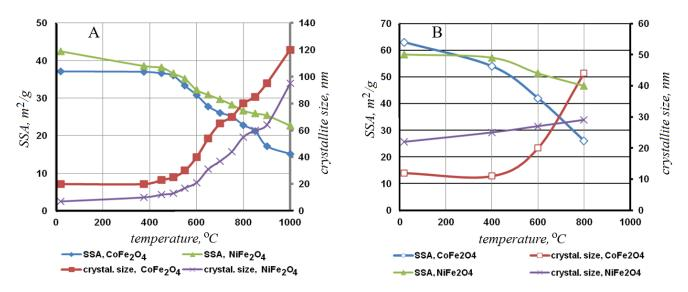
Fig. 4. Specific surface area (SSA) and crystallite size comparison depending on temperature for  $NiFe_2O_4$  and  $CoFe_2O_4$  synthesized by the sol-gel self-combustion (A) and the hydrothermal (B) method.
