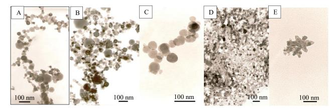
**Fig. 2.** The electron microscope image of  $CoFe_2O_4$  (A, C) and  $NiFe_2O_4$  (B, D, E) obtained by the plasma synthesis (A, B), self-combustion (C, D) and hydrothermal (E) methods.
