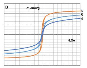
**Fig. 5.** The magnetic properties of the sample CoFe<sub>2</sub>O<sub>4</sub> prepared by the hydrothermal synthesis (A) after thermal treatment at 400 °C (1), 600 °C (2) and 800 °C (3) and NiFe<sub>2</sub>O<sub>4</sub> prepared by the self-combustion synthesis (B) after thermal treatment at 450 °C (4), 650 °C (5) and 850 °C (6).
