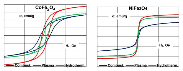
Fig. 3. Magnetic properties of ferrites synthesized by the sol-gel self-combustion and the hydrothermal method and in plasma.
