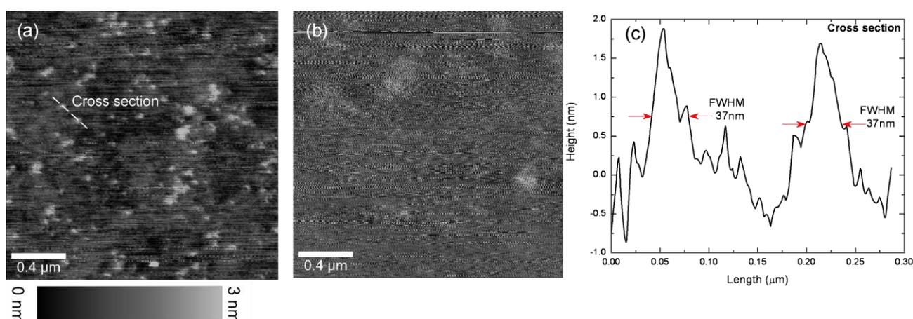
**Fig. 1.** (a) AFM image of silver colloid nanoparticles; (b) AFM image of glass substrate used for placing a drop of the colloid; (c) diagram for measuring the diameter and thickness of nanoparticles. The bar at the bottom of the figure shows a correlation between the thickness of a nanoparticle and the intensity of its grey colour in the image
