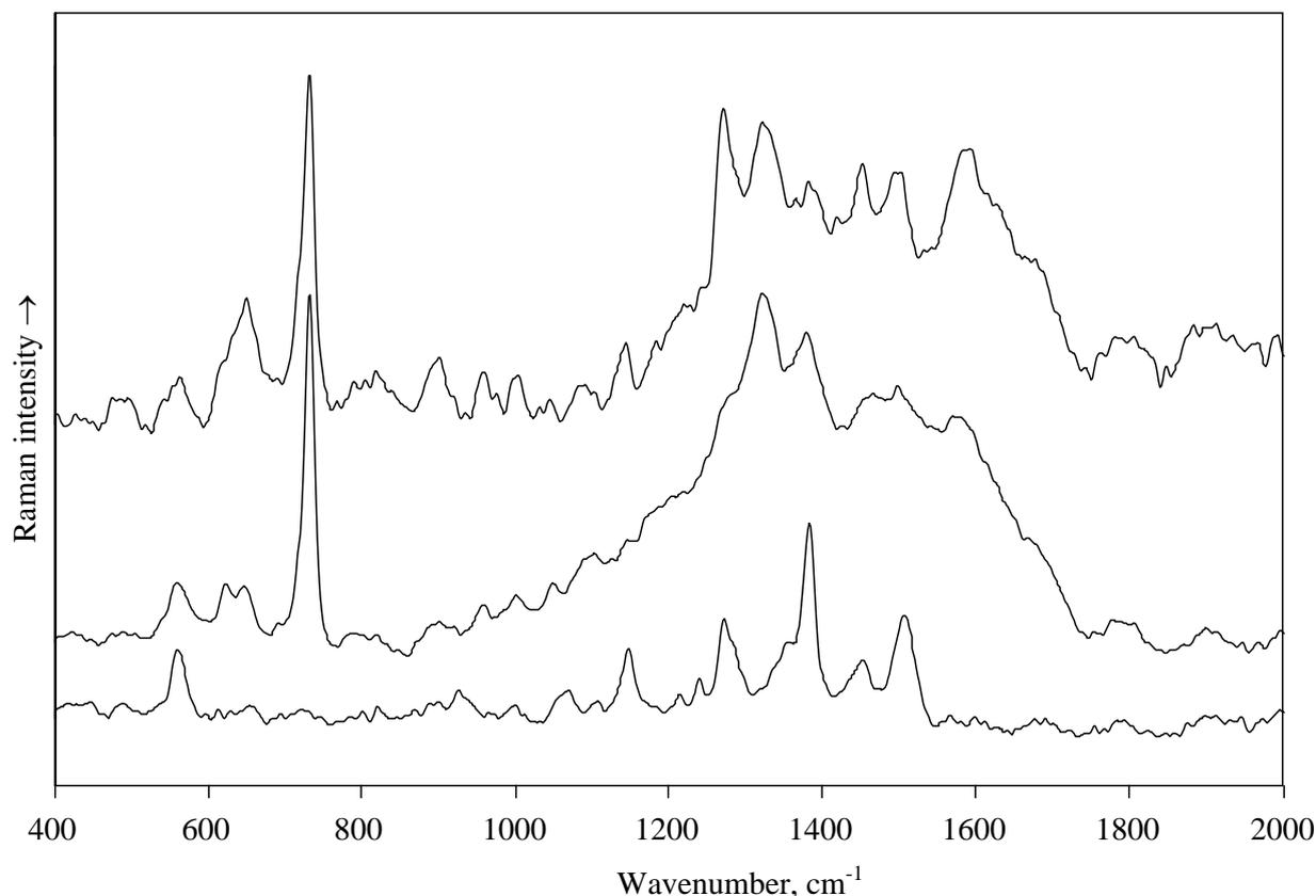
**Fig. 2.** SERS with NIR excitation (1064 nm) spectra of thermotolerant (top) and thermoresistant (middle) *Listeria monocytogenes* in the spectral region of 400–2000  $\text{cm}^{-1}$ . The bottom curve represents the Raman spectrum of the silver colloid
