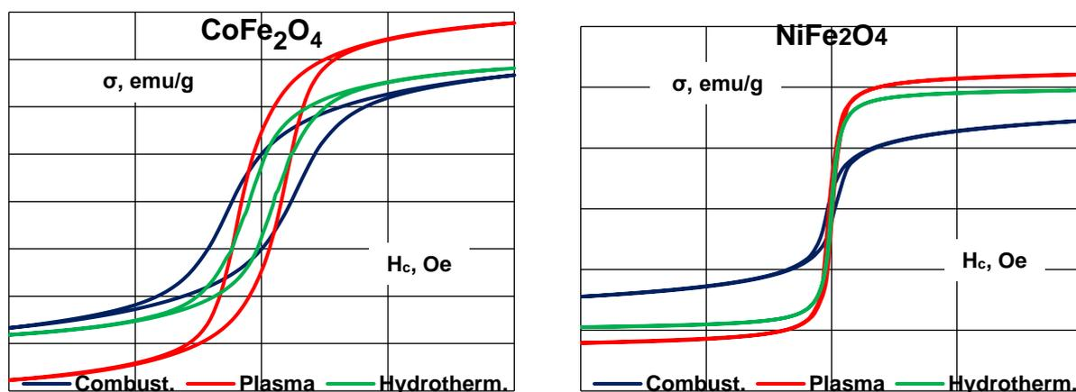
**Fig. 3.** Magnetic properties of ferrites synthesized by the sol-gel self-combustion and the hydrothermal method and in plasma.
