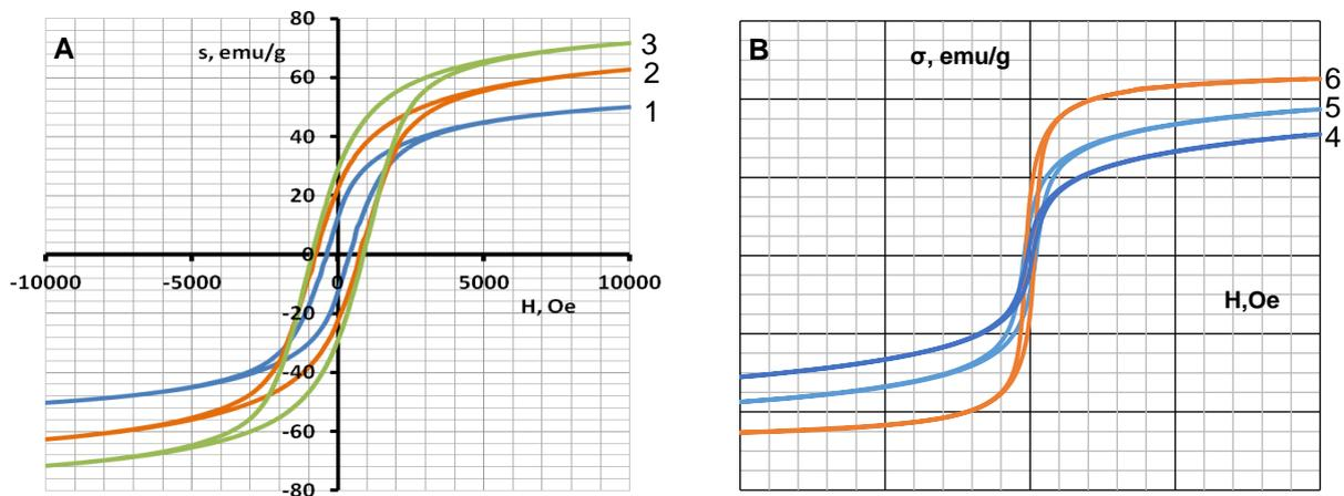
**Fig. 5.** The magnetic properties of the sample CoFe<sub>2</sub>O<sub>4</sub> prepared by the hydrothermal synthesis (A) after thermal treatment at 400 °C (1), 600 °C (2) and 800 °C (3) and NiFe<sub>2</sub>O<sub>4</sub> prepared by the self-combustion synthesis (B) after thermal treatment at 450 °C (4), 650 °C (5) and 850 °C (6).
