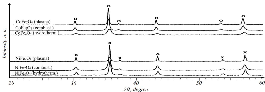
**Fig. 1.** XRD pattern of ferrite nanopowders: o – CoFe<sub>2</sub>O<sub>4</sub>, x – NiFe<sub>2</sub>O<sub>4</sub>.
