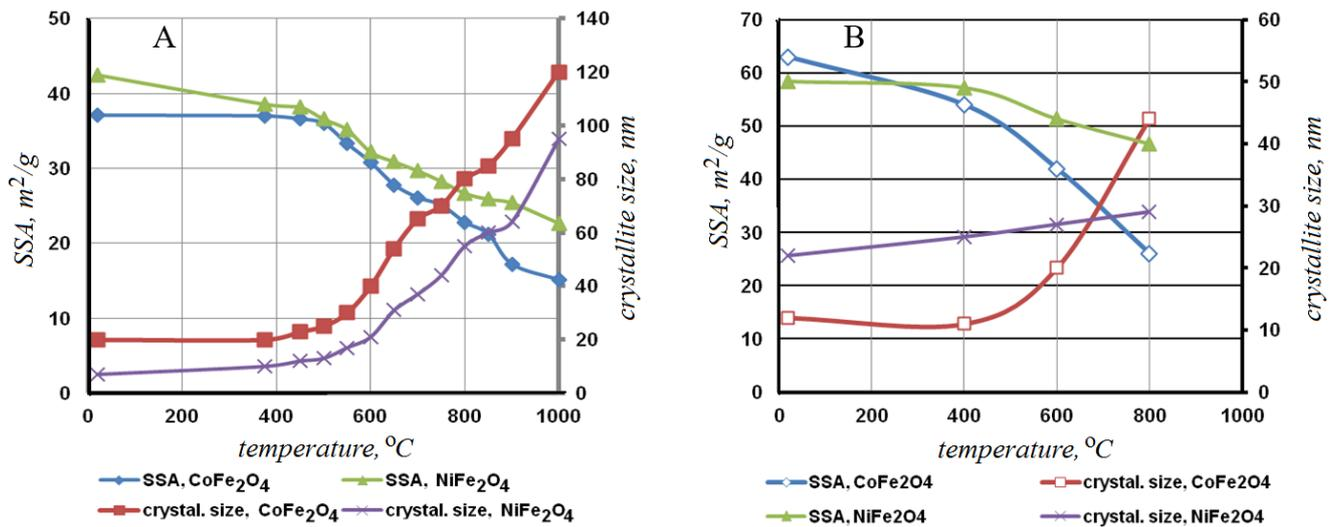
**Fig. 4.** Specific surface area (SSA) and crystallite size comparison depending on temperature for NiFe<sub>2</sub>O<sub>4</sub> and CoFe<sub>2</sub>O<sub>4</sub> synthesized by the sol-gel self-combustion (A) and the hydrothermal (B) method.
