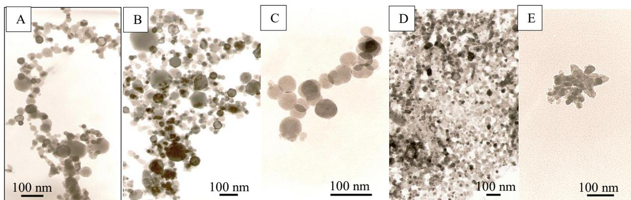
**Fig. 2.** The electron microscope image of CoFe<sub>2</sub>O<sub>4</sub> (A, C) and NiFe<sub>2</sub>O<sub>4</sub> (B, D, E) obtained by the plasma synthesis (A, B), self-combustion (C, D) and hydrothermal (E) methods.
